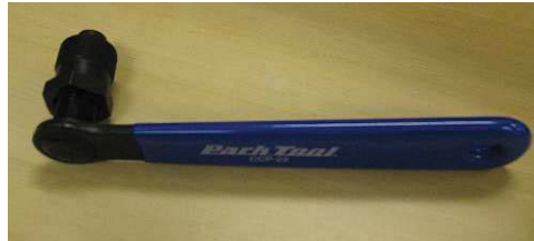
Diagram 7.6 - Park Tool CCP-22 Crankarm Puller
